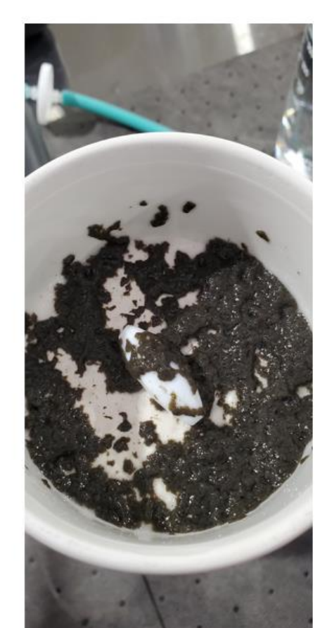
Stop Vacuum Filtration timing when reach 50 mL filtered Measure turbidity and TSS of the filtrate
